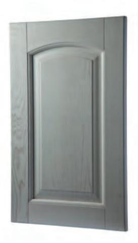
Solid ash panel door. Worked panel in solid ash. At tenoning assembled. White pickled lacquered finish.
