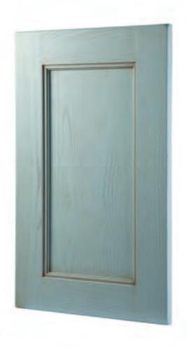
Solid ash panel door. Flat panel in chipboard veneered with ash. At tenoning assembled. Blue lacquered finish with decapè.
