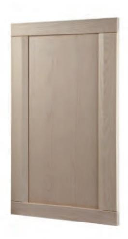
Solid ash panel door. Flat panel in chipboard veneered with ash. Natural matt finish.
